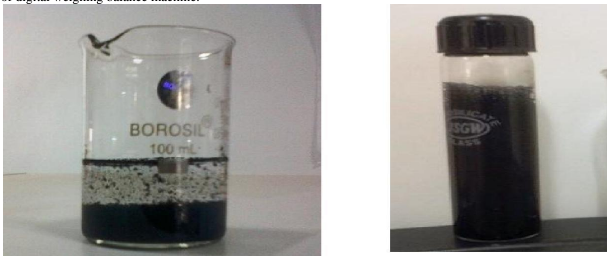
Fig. 2.1 the prepared CNT/water HT fluid without using any Surfactant and with using Surfactant Respectively
